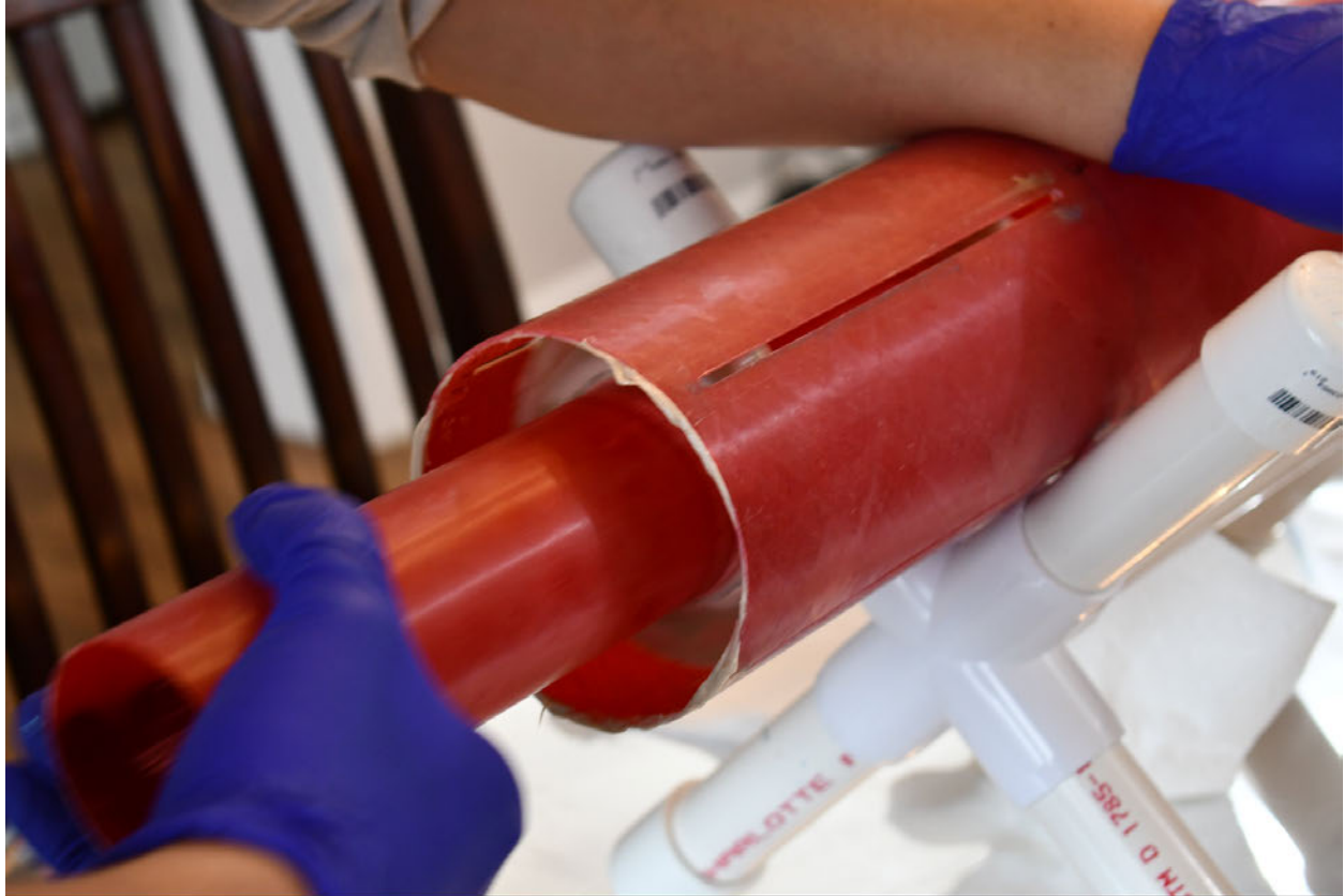
Image 14: Installing the motor tube into the airframe.
