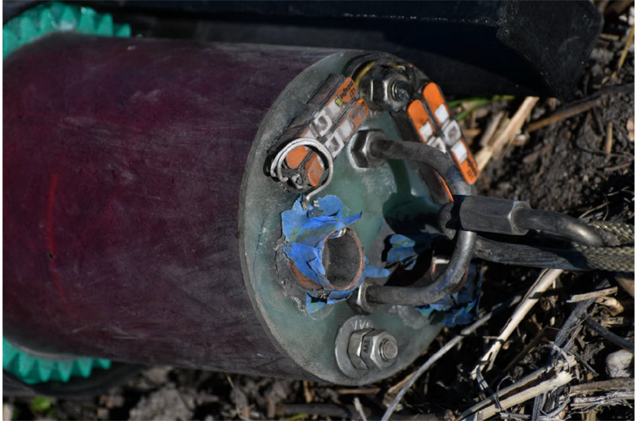
Image 36: Drogue ejection charges post-flight
