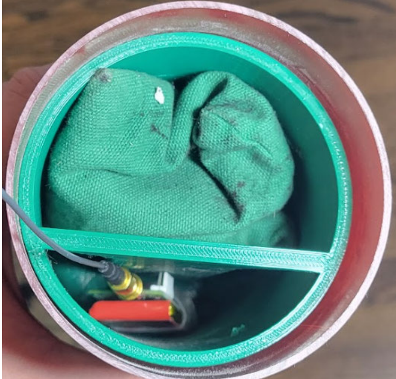
Image 26: GPS Tracker in the nose cone sled (not in flight-ready configuration)
