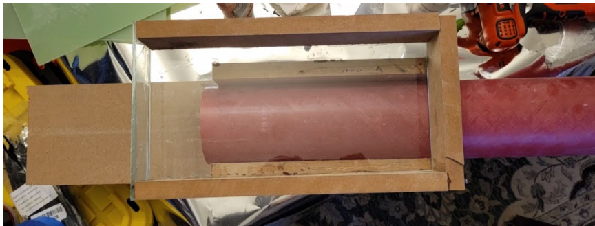
Images 2 & 3: Custom-built jig used to cut fin slots
