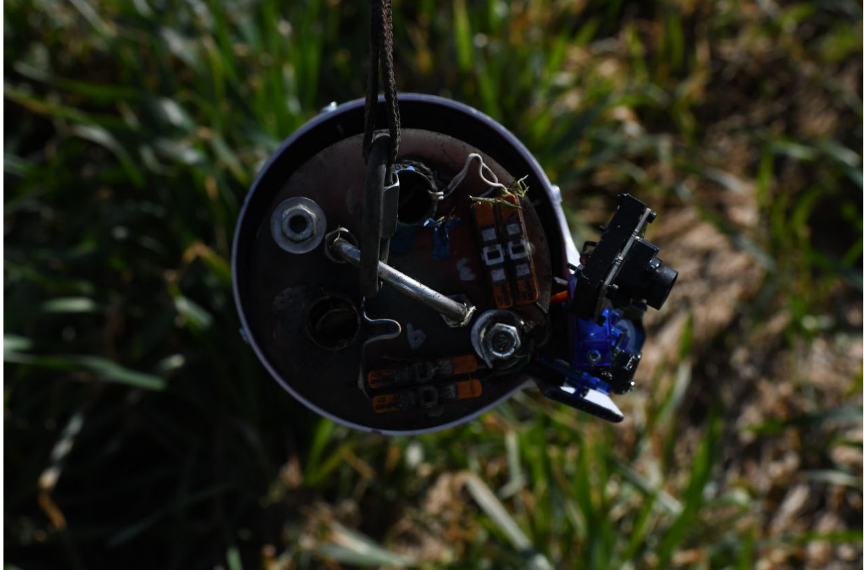
Image 58: Drogue ejection charges after flight
