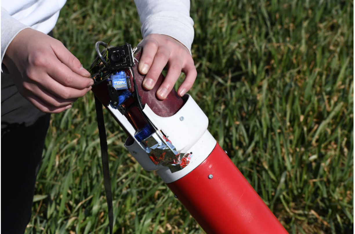
Image 47: Image showing the damaged payload arm housing and the retention of hardware components.
