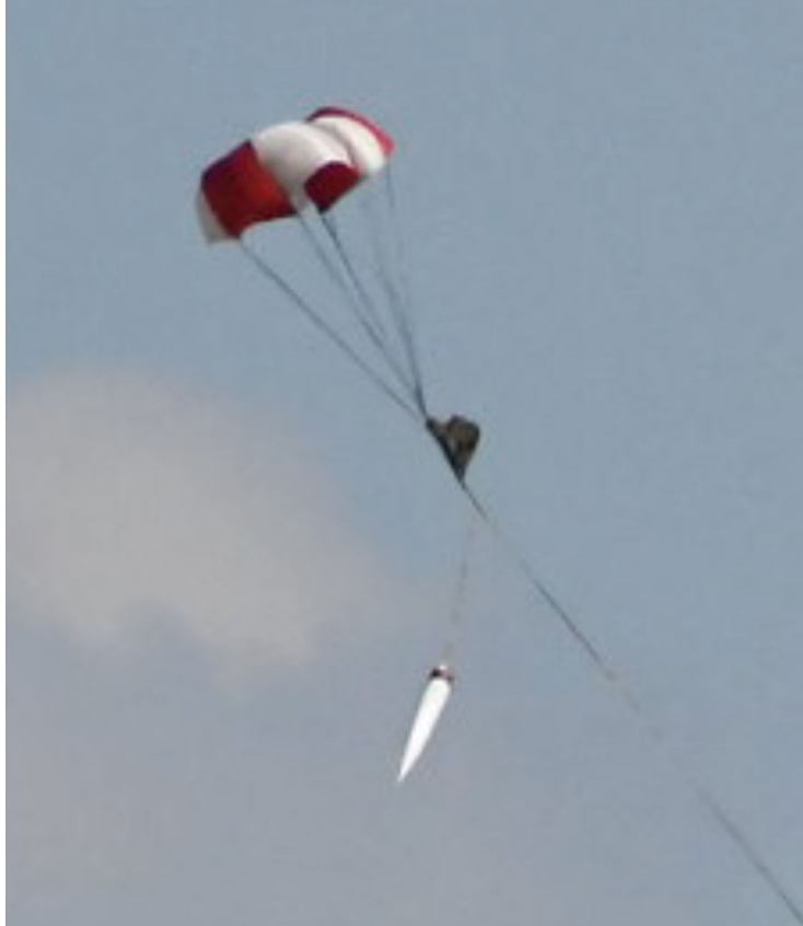
Image 50: Image of the main parachute, the spill hole line is shown on the right side of the parachute.
