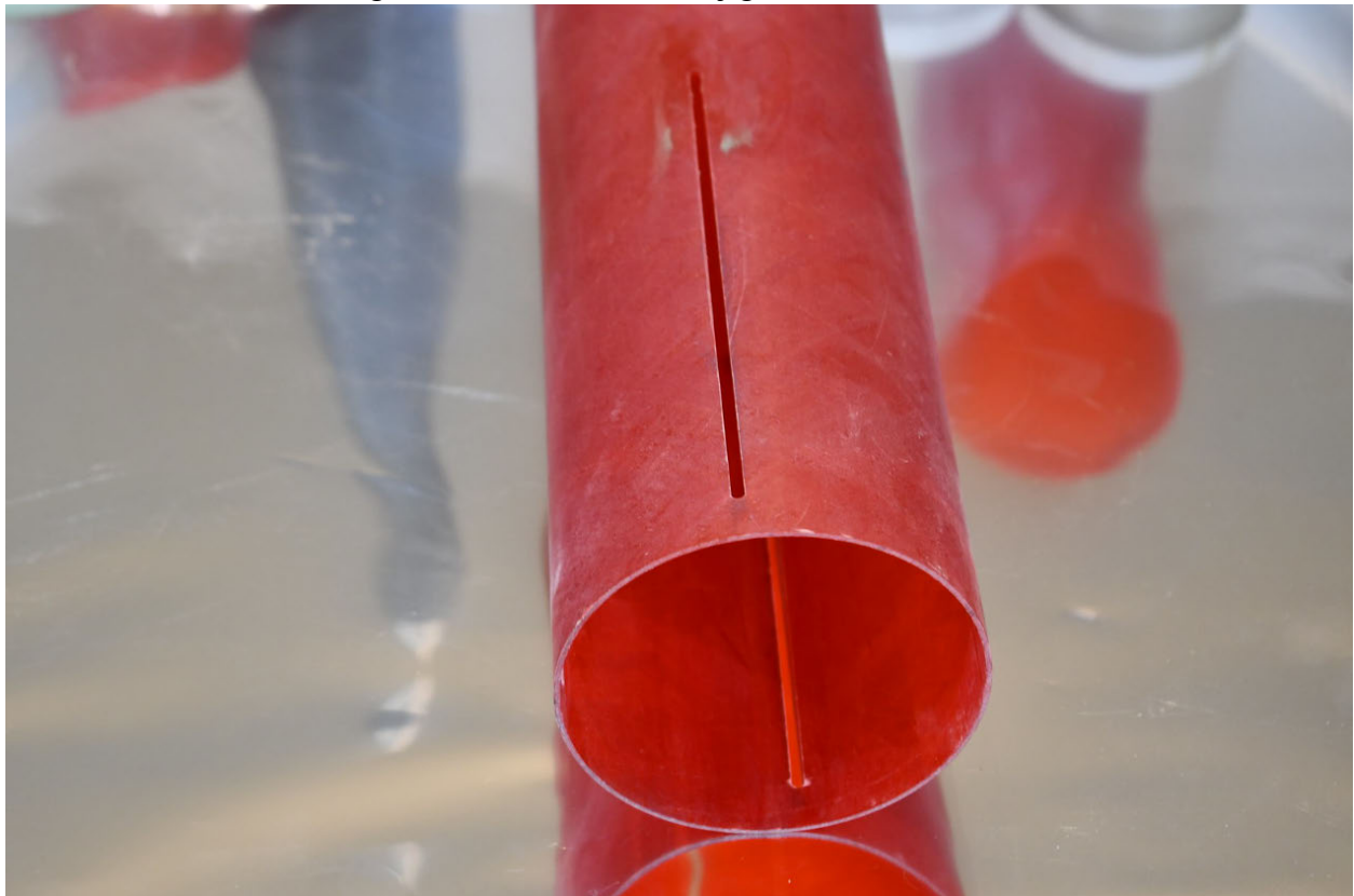
Image 4: Body tube fin slots, cut and sanded with labels corresponding to fins that best fit in the slot.
