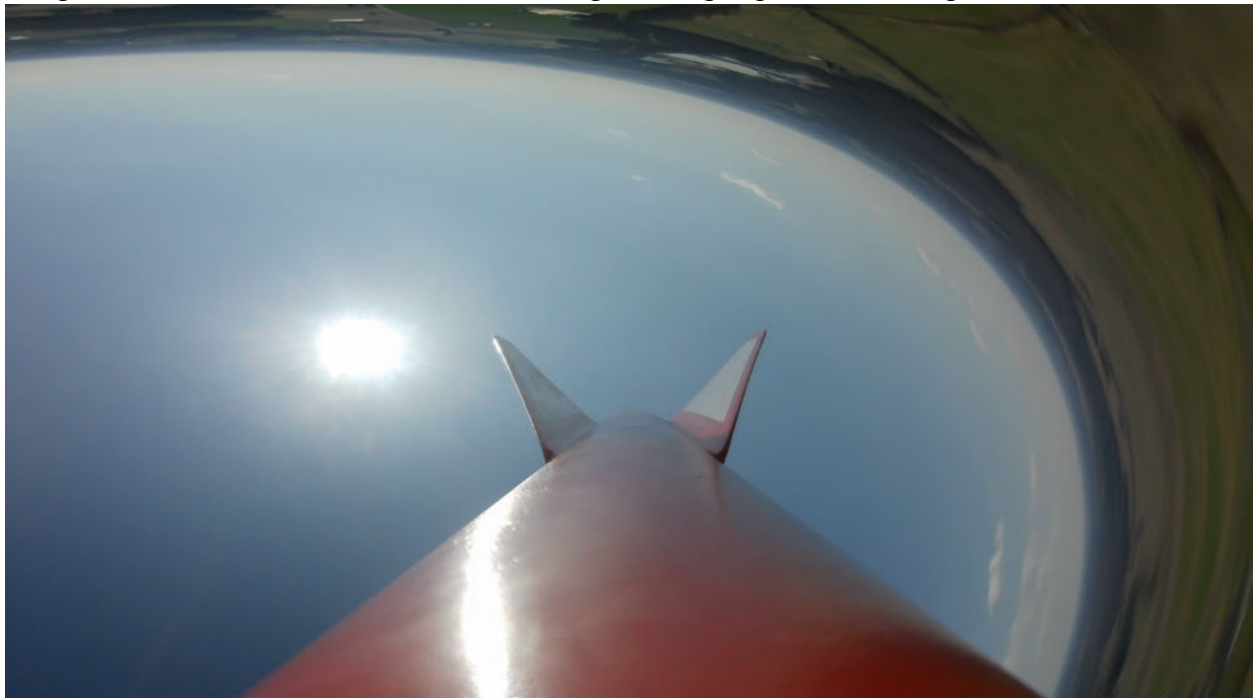
Image 41: Frame from Runcam video shortly before landing showing distortion in the video caused by spinning
