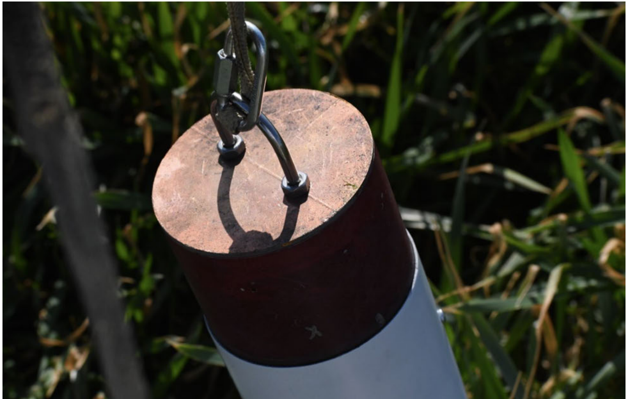
Image 22: Nose cone bulkhead as configured for flight.
