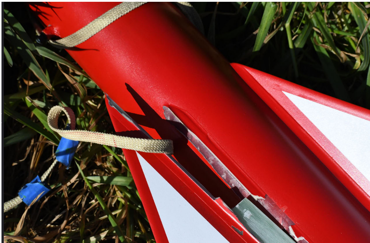
Image 45: Close up of fin damage as found
