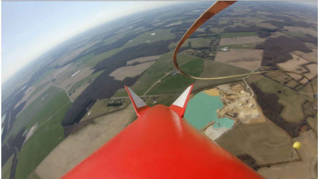
Image 40: Frame from Runcam video showing the drogue parachute being below the fin section.
