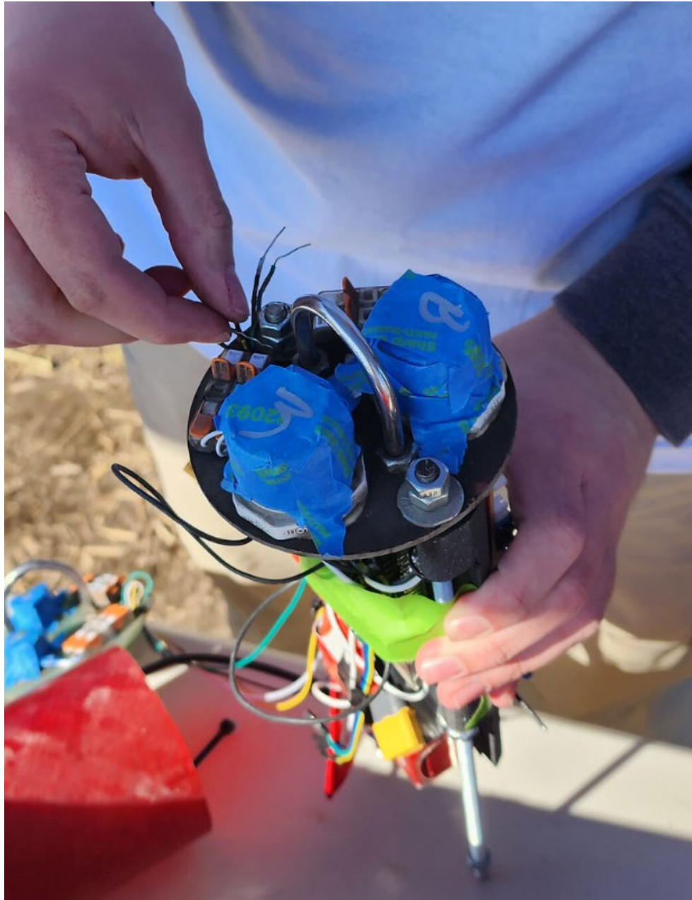
Image 20: Forward (main parachute) avionics bay bulkhead as prepared for flight.
