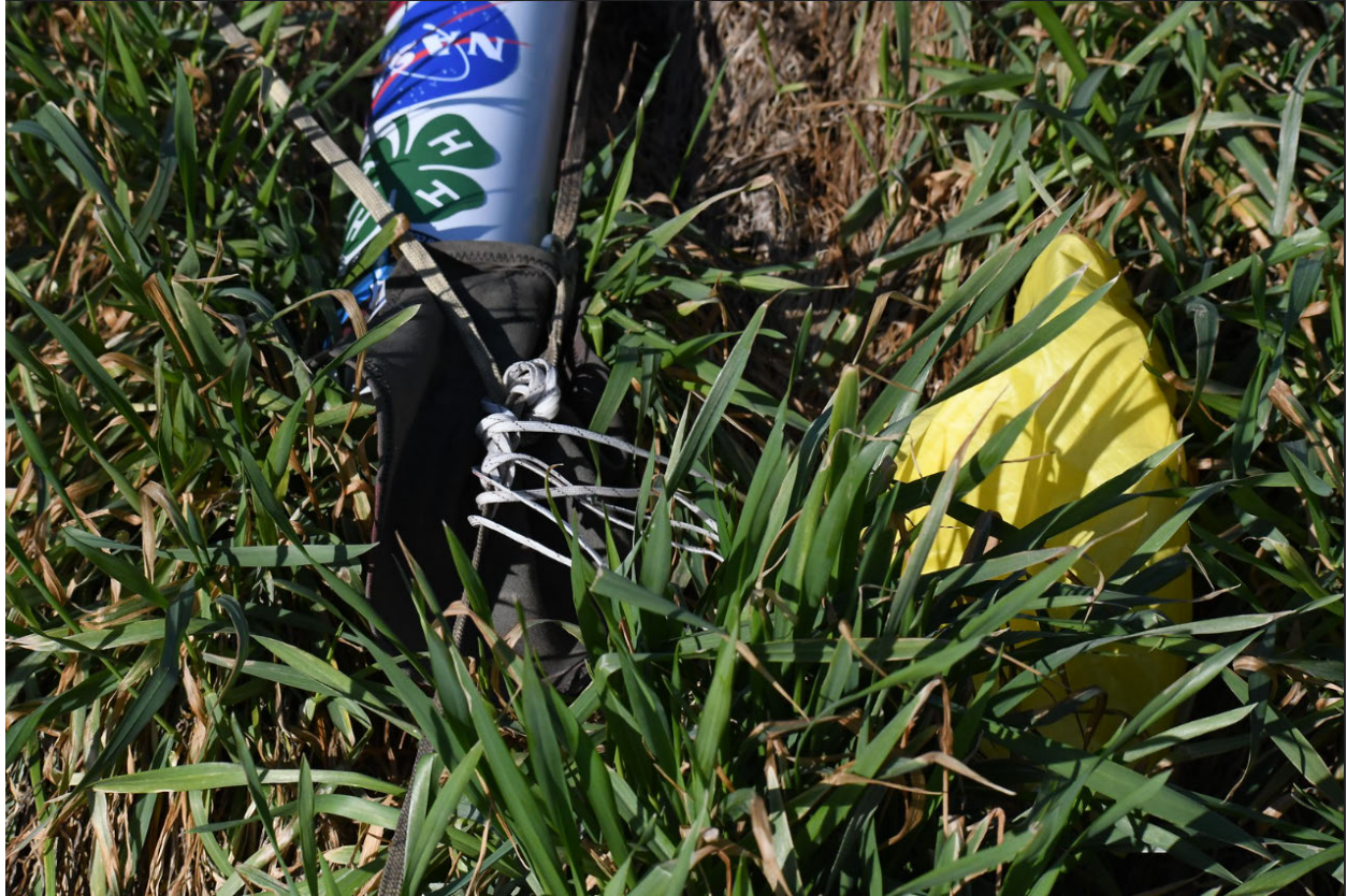
Image 56: Drogue parachute tangled at base of main parachute shock cord
