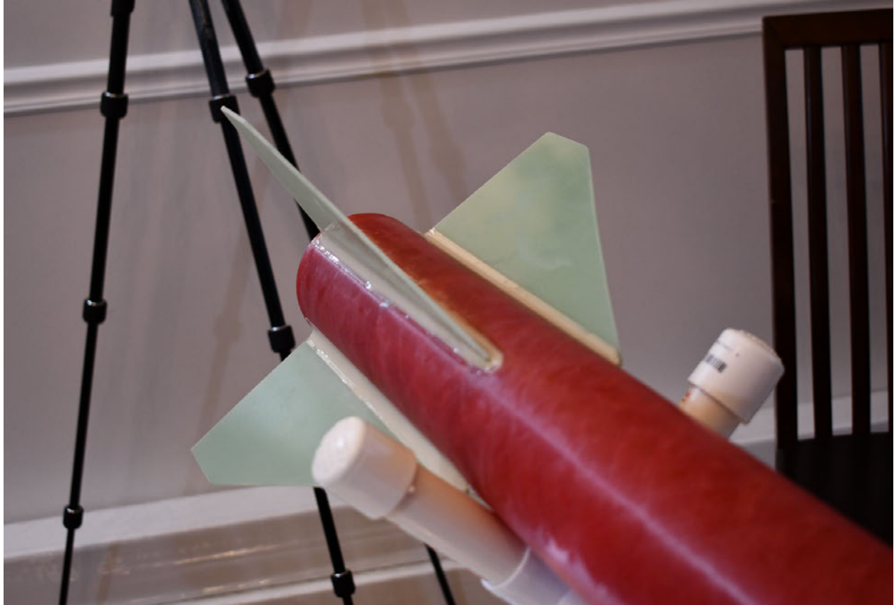
Image 19: Fillets cleaned and tape removed.
