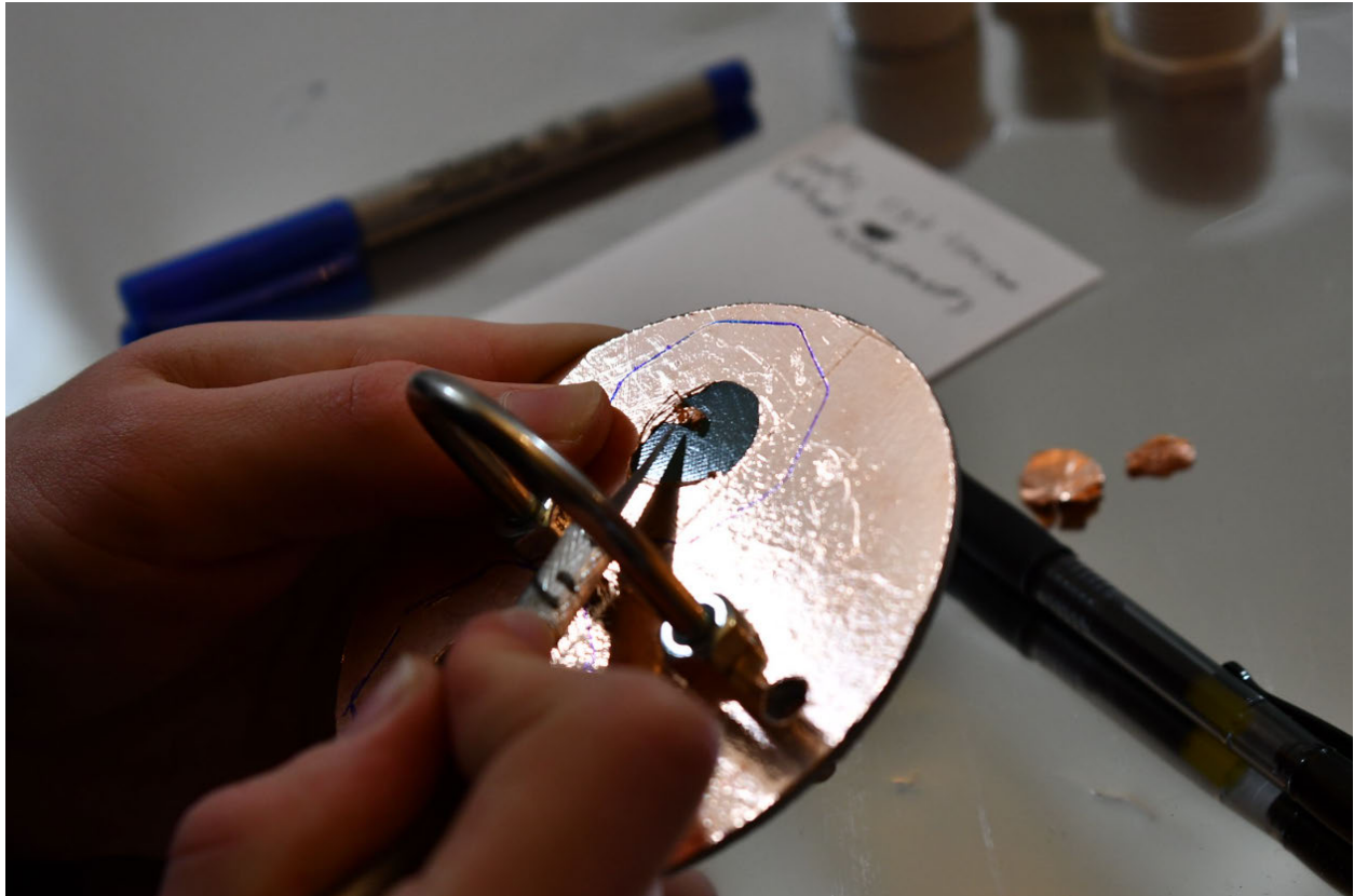
Image 20: Clearing an area on the forward avionics bay bulkhead for charge wells.
