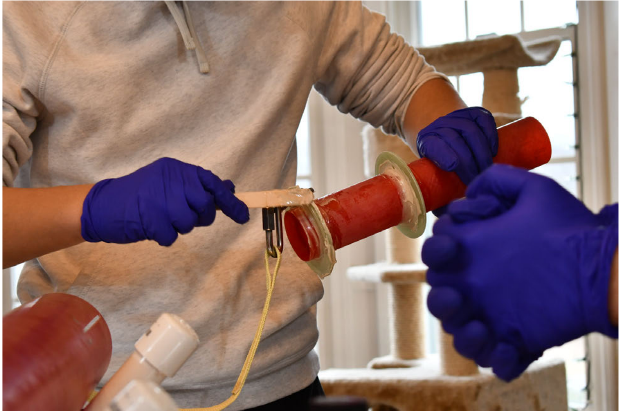
Image 13: Epoxying centering rings before installation to the airframe.
