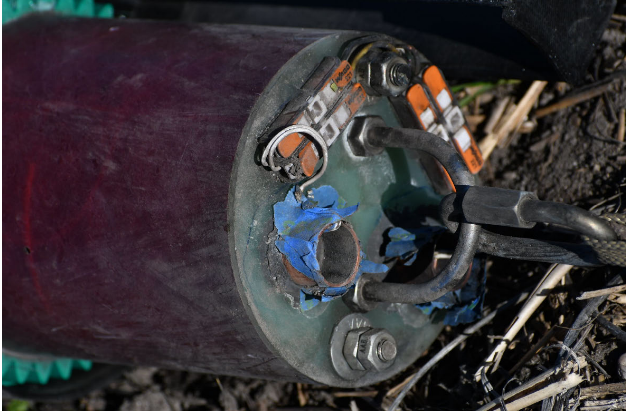
Image 21: Aft (drogue parachute) avionics bay bulkhead as built
