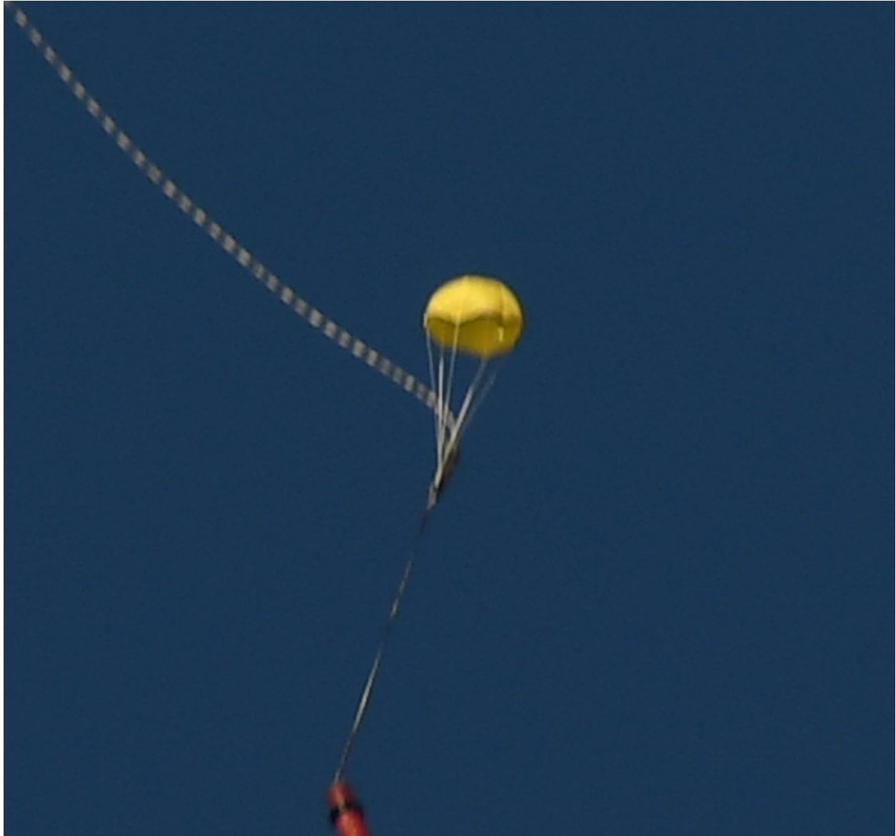
Image 39: Image of the drogue parachute and lines shortly after drogue parachute deployment.
