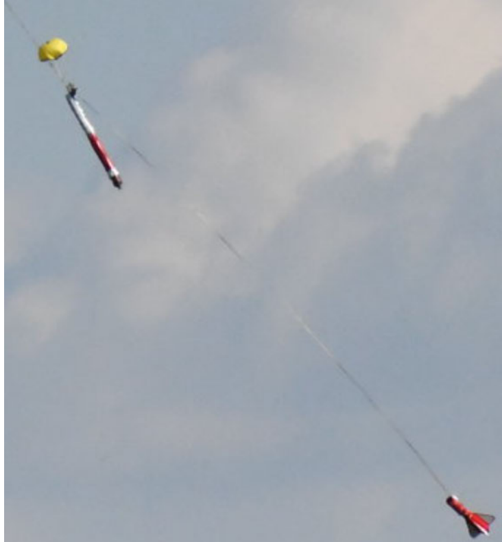
Image 42: Image showing the entanglement of the drogue parachute after main parachute separation.
