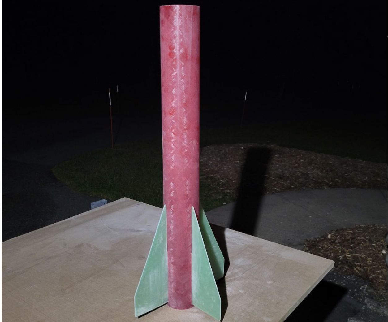
Image 6: Dry fit of slotted body tube, fins, and cut body tube.
