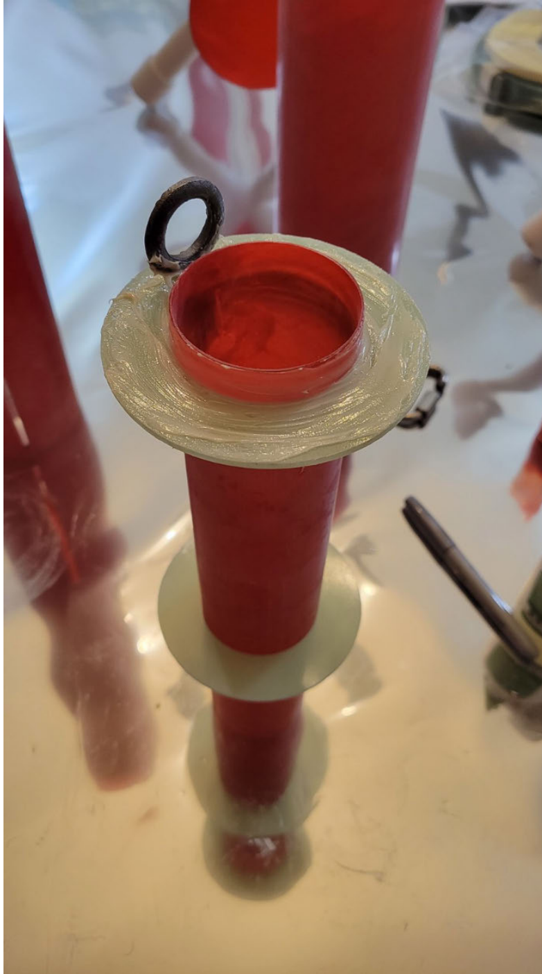
Image 7: Motor tube with eye-bolt and top two centering rings epoxied
