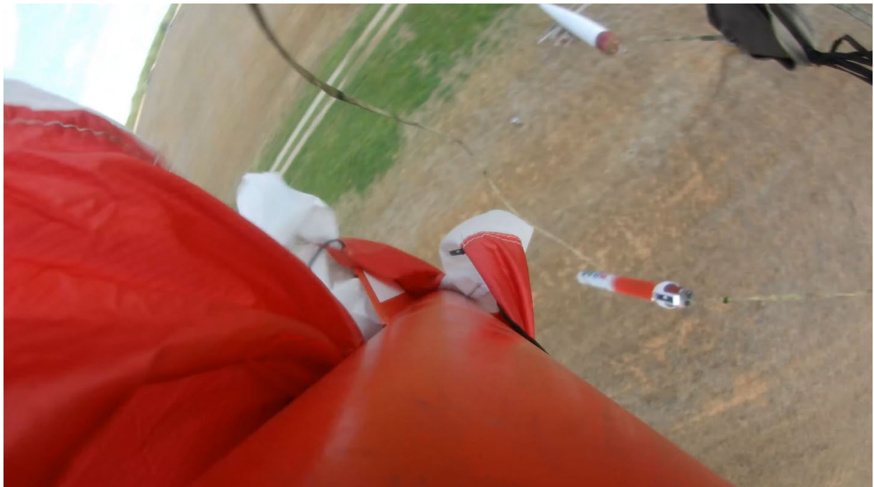
Image 5. Picture from onboard video of the sustainer making contact with the main parachute
