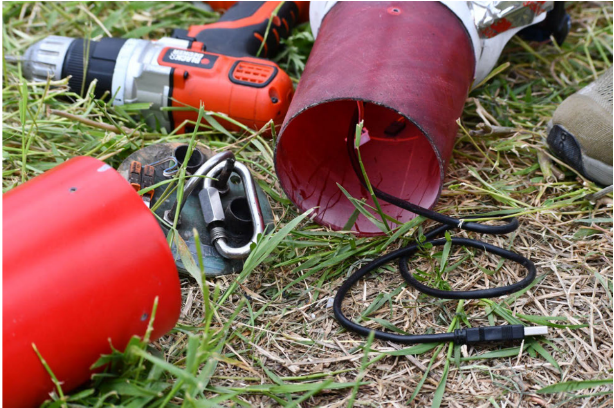
Image 12. Soot inside of avionics bay coupler (at altitude check)
