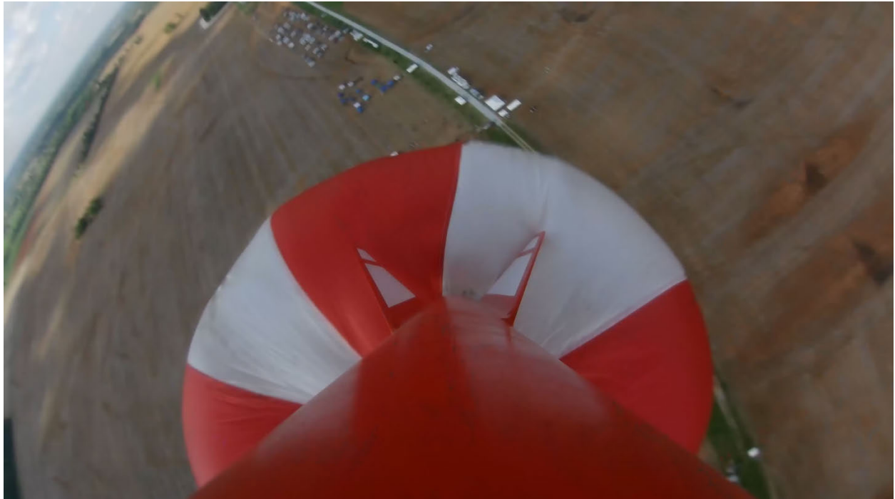
Image 5. Picture from onboard video of the sustainer making contact with the main parachute
